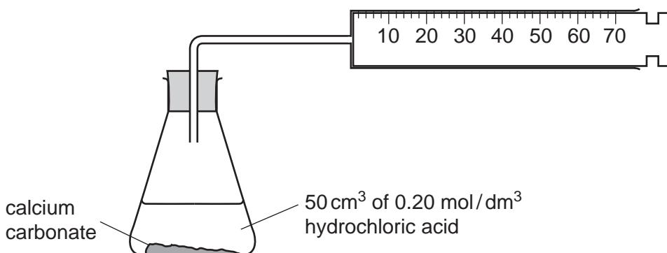
The diagram below shows the gas syringe containing the volume of carbon dioxide collected in one minute.
